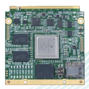
*i*Wave systems launching high performance Q7 SOM module based on Freescale's i.MX6x ARM Cortex-A9 processor for faster and multimedia focused applications. With extreme peripheral integration, the CPU supports industry latest high-performance interfaces, such as PCle Gen2, Gigabit Ethernet, SATA 3.0, HDMI 1.4, SDXC, MIPI CSI/DSI and 64-Bit DDR3 interfaces.
